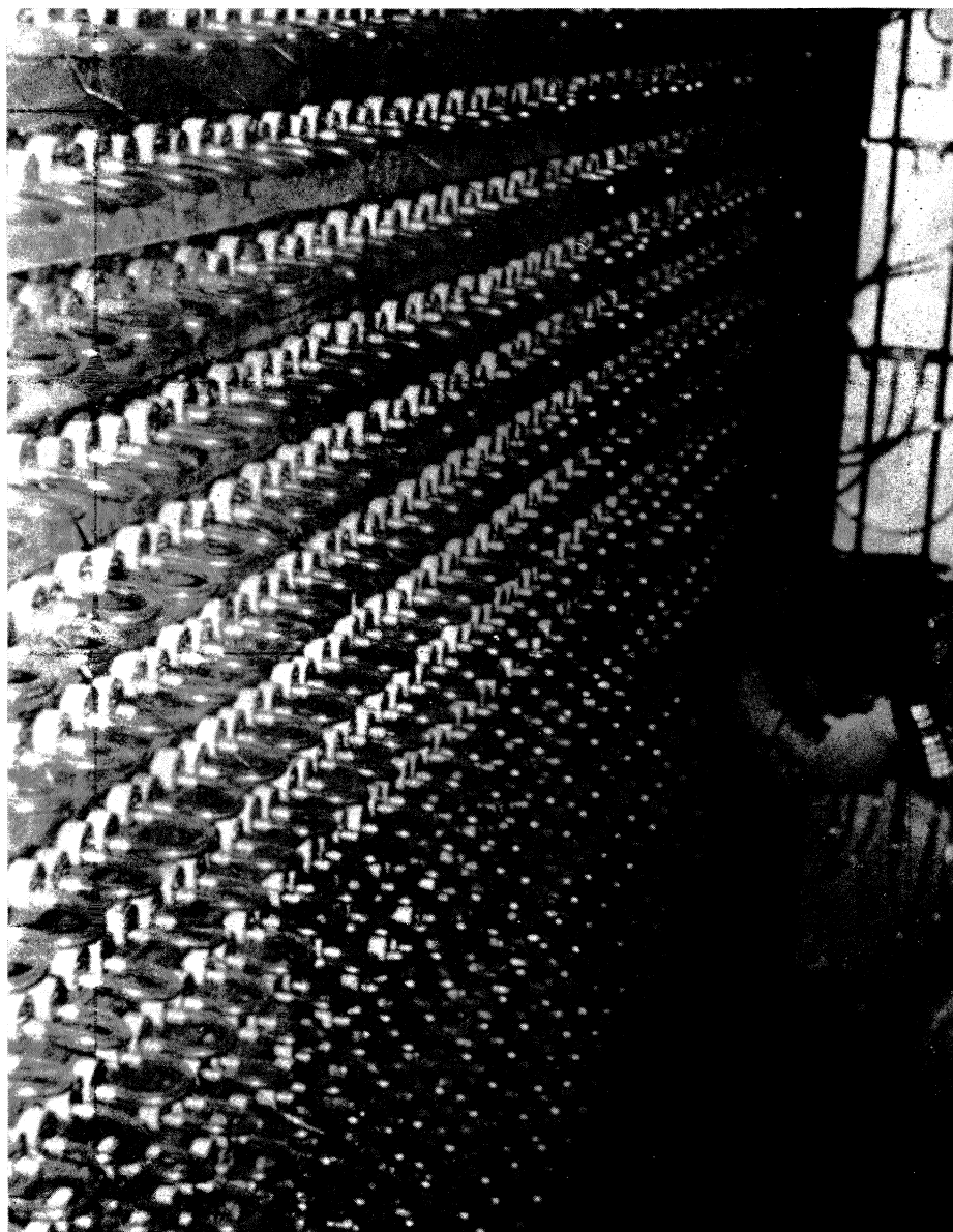
Inspecting the Soudan 1 underground detector prior to the installation of the electronics. The ends of some of the 3456 gas proportional tubes can be seen protruding from the iron-loaded concrete calorimeter material.
